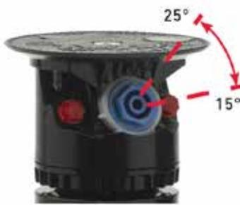
The 25° setting provides maximum distance of throw and the 15° setting provides improved wind performance, radius reduction and obstacle avoidance.
