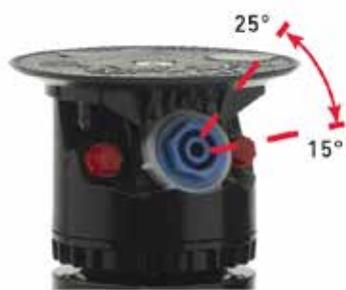
The 25° setting provides maximum distance of throw and the 15° setting provides improved wind performance, radius reduction and obstacle avoidance.
