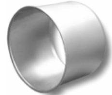
HDPE internal stiffeners are formed of stainless steel to the actual inside diameter of the pipe. They are recommended for all HDPE pipe end connections utilizing bolt on fittings (excluding saddles) to prevent pipe contraction during temperature changes.
