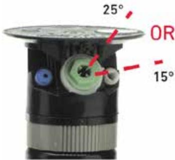
The 25° setting provides maximum distance of throw and the 15° setting provides improved wind performance, radius reduction and obstacle avoidance.
