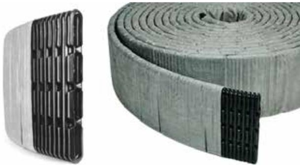
A perforated panel-shaped polyethylene core in 12" and 18" widths and in coils up to 100'. Can be used with or without a covering geotextile sock for filtration of fines. 12" AdvanEDGE has twice the response rate of 4" round pipe, removing a given quantity of water 60% faster. AdvanEDGE can be installed vertically in narrow trenches for field and perimeter drainage, or laid flat directly on the subgrade of greens and bunkers.
