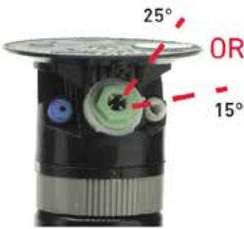
The 25° setting provides maximum distance of throw and the 15° setting provides improved wind performance, radius reduction and obstacle avoidance.
