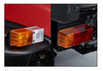
Signal Light Kit • Brake, tail and turn signals are integrated into one optional kit
