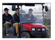
Windshield For Canopy • Quick and easy to fold down to allow air flow and enhance operator comfort
