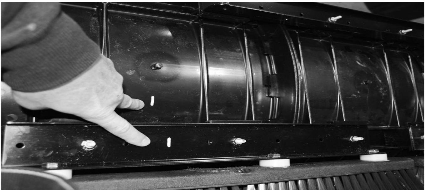
**STEP 3:** Attach the travel brackets to the ProCore by drilling out the top hole of the bracket as shown with a 1/4" bit - be careful not to drill into the plastic cover. Attach the bracket as shown in the lower picture - nylon locking nut on the inside. Do not over tighten - allow for the bracket to swing freely.
