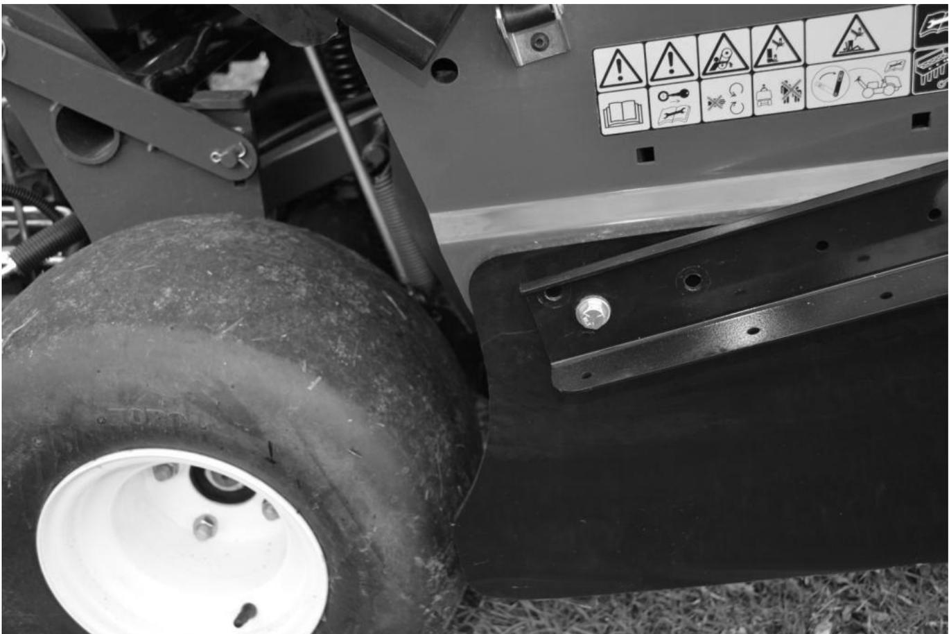
**STEP 5:** Lift the blade into the resting brackets. Insert the 3inch 3/8" bolt along with the 4 nylon spacers into the back hole and tighten securely. For security, attach a bungee cord or strap while in this travel position. Carefully lower the Core Collector until it rest on the bolts with the spacers.
