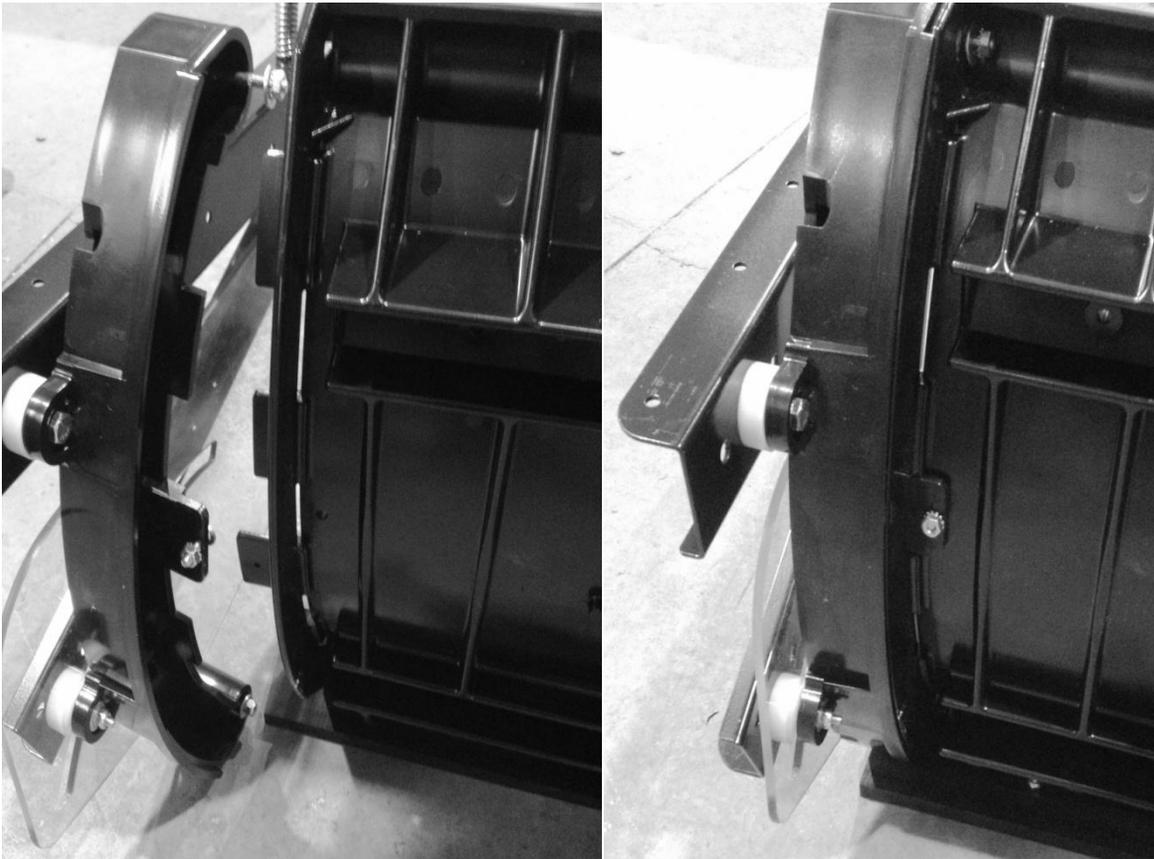
**STEP 2:** To attach the brushes, place the blocks as shown with the smooth ridge facing down. Place brush channel against blocks and tighten the screws. Note that there is a right and left side to the brush channel.
