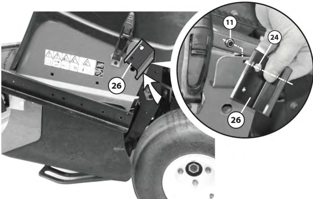
**STEP 4:** Remove the bolts holding the side panel of the Procore 648 and save. Attach the end of the side arms into the hole closest to the wheel as shown. Be sure to use the nylon locking nuts. Tighten securely but allow for some rotation of the arm.
