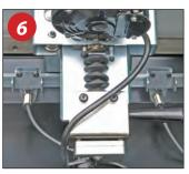
**Proximity Switches:** Durable traverse proximity switches are easily positioned to control the length of travel for the grind area. These allow for the fast repetitive set-up for identical blades, producing a perfect consistent grind each and every time.
