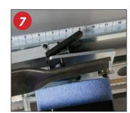
Blend Radius Relief Slide Bar: The measuring decal associated with the relief slide bar makes the set-up process extremely fast. This is one of the many features that makes the repeatability of set-up so easy, reducing the amount of time to change from different blade types to mere seconds.
