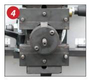
Center Hole "Quick Connect Cone": With the push of a button, a cone-shaped mount slides on a threaded stud to securely mount the blade's center hole in the mounting fixture.
