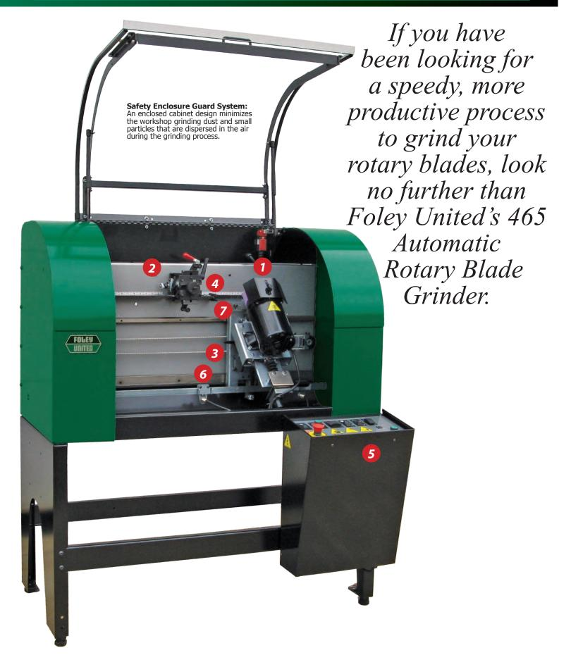
Foley United's NEW 465 Automated Rotary Blade Grinder is the most innovative product to enter the Turfcare Industry in years! The enclosure system for dust and noise, time savings, and the ability to reproduce the OEM grind surface are only a few of the many benefits that the 465 offers. The unique design of the 465 features automated infeed cycles and a built-in blade balancing system that makes the grinding process safer and more efficient than ever thought possible!
