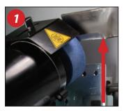
**OEM End of Grind Blend Radius:** A key feature of the 465 is an ability to produce the blend radius that is engineered into all new blades. This unique patented feature minimizes blade stress that can be common with other rotary blade grinding systems and produces a blend-out that is consistent, safe, and effective.
