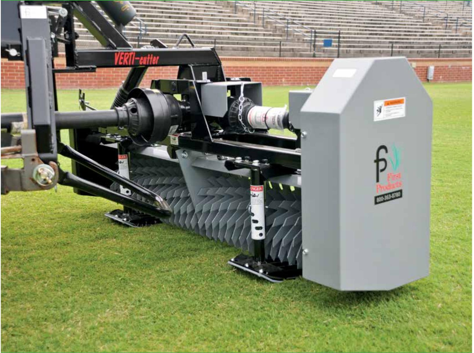
The depth gauge skids are directly centered under the shaft allowing the skids to float over undulations without losing depth. The skids are preferred in southern type turfs such as Bermuda and zoysia. The replaceable skids systems are made of durable polypropylene.
