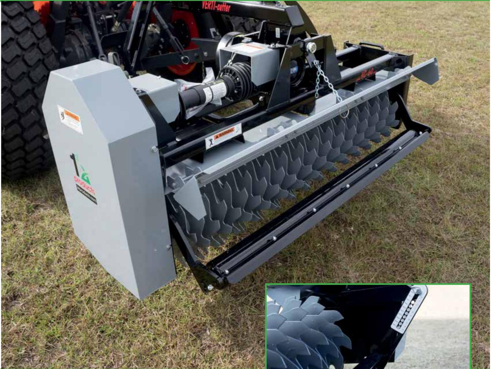
The double roller depth gauge system allows for consistent depth control over undulations. The roller offers two big improvements, it prevents marring of the turf and eliminates the forward and rear edge of the skids from digging or pushing up turf which is common in bent grass. With rollers, you can have the option for 1.5" spacing. The rollers are favored in northern turf such as bent grass
