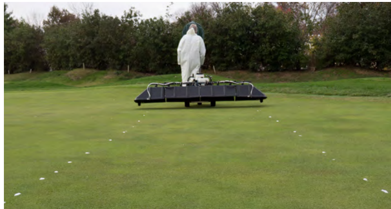
New! A custom foam marking kit is available to accurately line-up for each pass and helps to assure accurate overlap.
