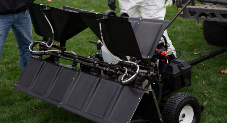
The outer wings and the handle fold up for compact transport.
