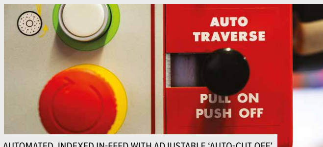
AUTOMATED, INDEXED IN-FEED WITH ADJUSTABLE 'AUTO-CUT OFF'
