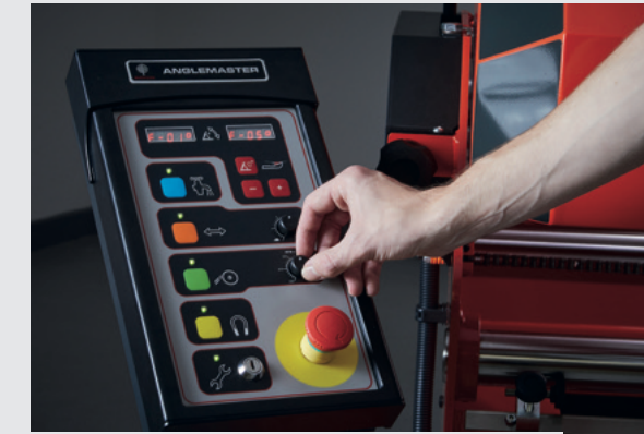
EASY TO USE CONTROL PANEL WITH DIGITAL ANGLE FINDER
