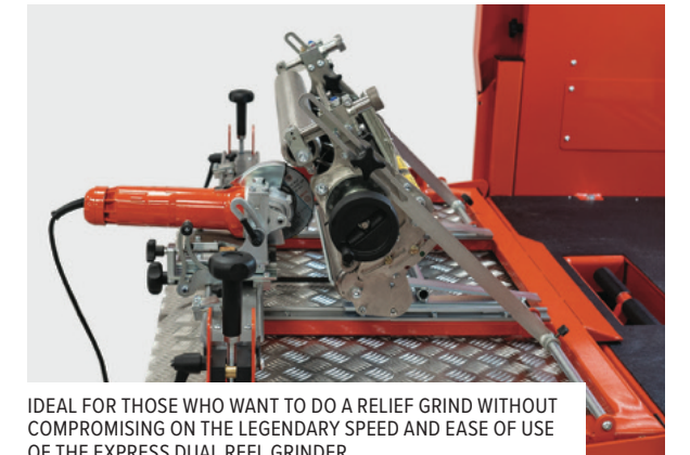
THE CARRIAGE DESIGN GIVES GREATER STABILITY AND INCREASES THE ACCURACY FOR RELIEF GRINDING
