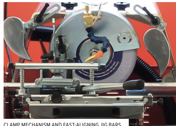
CLAMP MECHANISM AND FAST-ALIGNING JIG BARS
