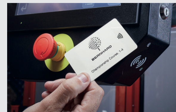
RFID TECHNOLOGY FOR RECALL OF PROGRAMMES AND ACCESS USER PREFERENCES
