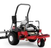
Sand Pro 2040Z The Sand Pro 2040Z is a unique zero-turn mechanical ball field groomer that delivers unmatched maneuverability and productivity. The exclusive nail drag/flex groomer with "Lift in Turn" feature, makes the inside flex tooth rake section lift in a tight turn preventing teardrop formation, leaving a uniform ball field surface.
