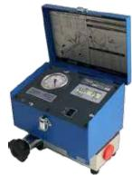
hydraulic system to test pumps, motors, valves and cylinders in both flow directions.
