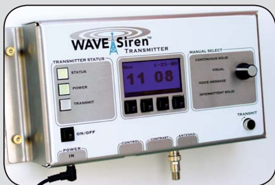
WAVE Transmitter sends signal to Sequencers.
