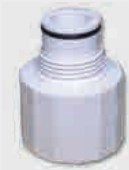
1 1/4" Female ACME x 1" Male ACME Adapter Allows you to upgrade existing Rain Bird® Eagle™* 700 1 1/4" sprinklers to any Toro 800S or DT Series Sprinkler. P/N TA36-132
