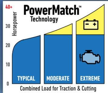
**Exclusive Hybrid Drive System** – PowerMatch technology enables the Reelmaster 5010-H to seamlessly match the power generated to the power required for traction and cutting based on the mowing conditions.
