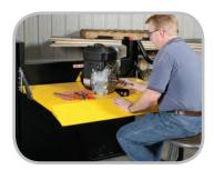
The Workstation will raise from a lowered floor position up to a height of 39.5" (100 cm).
