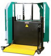
The Workstation can be used to transfer reels into a grinding machine, and can easily be put into a stored position.
