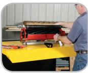
Setting heights-of-cut, making adjustments, and doing other reel work is made easier when the units are off the ground and at a friendly work height.
